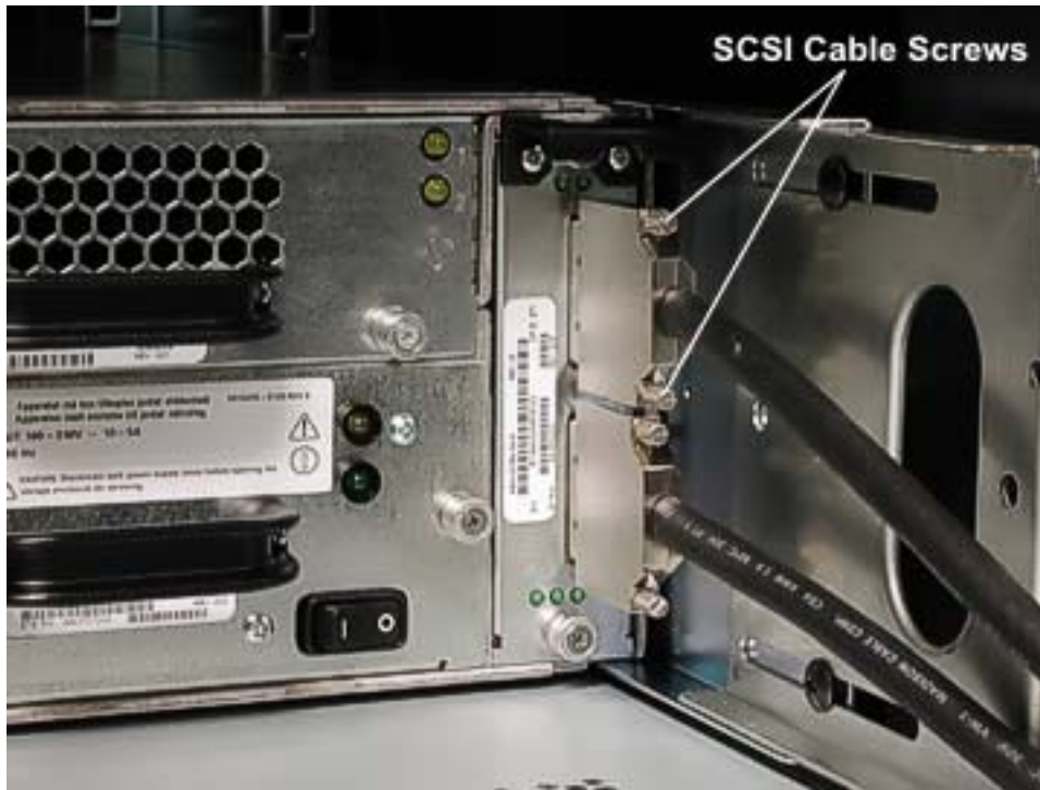
Figure 3-59. Captive Screws on SCSI Cable Connector at Enclosure
