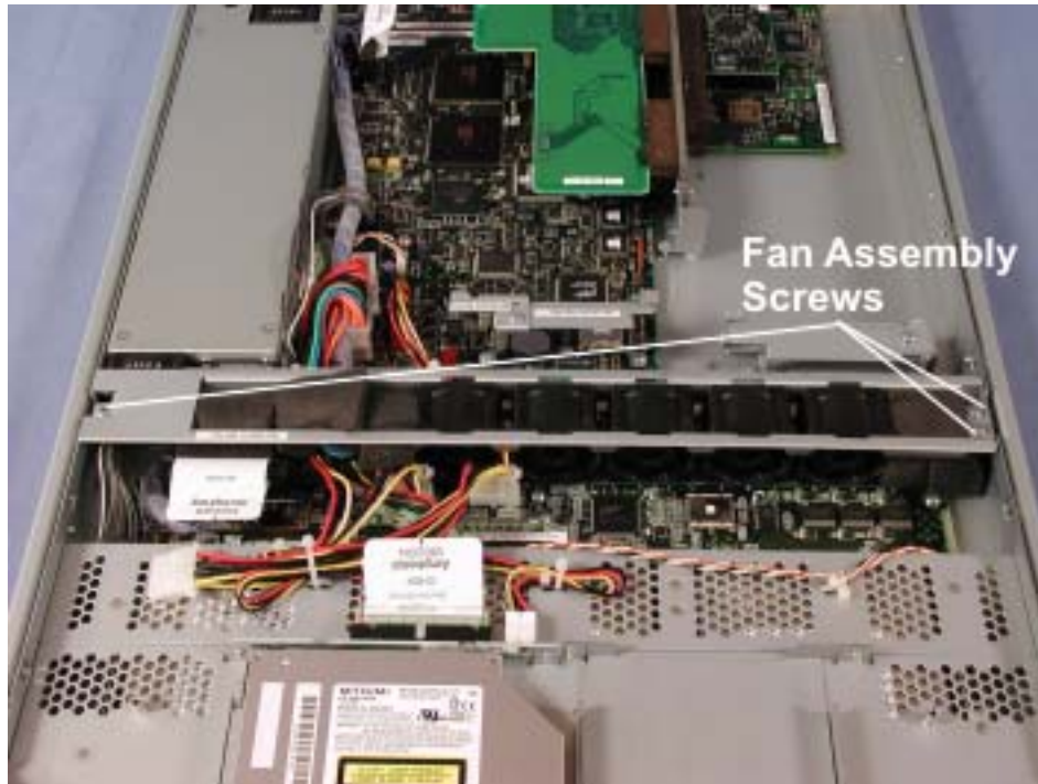
Figure 4-68. Fan Assembly Screws
