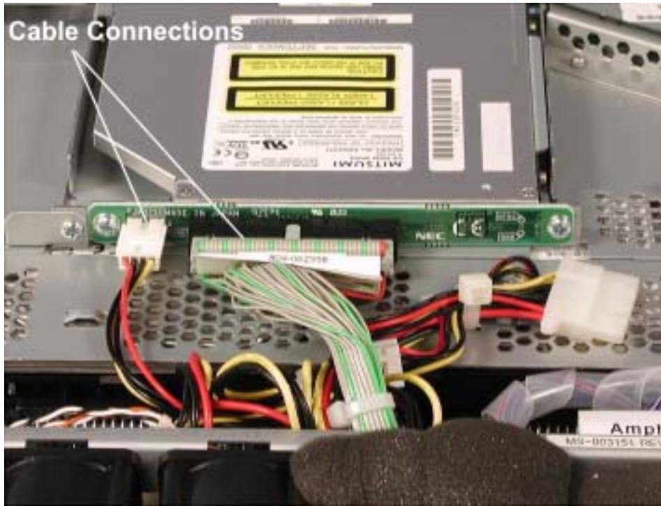
Figure 4-50. CD-ROM Interface Board Cables
