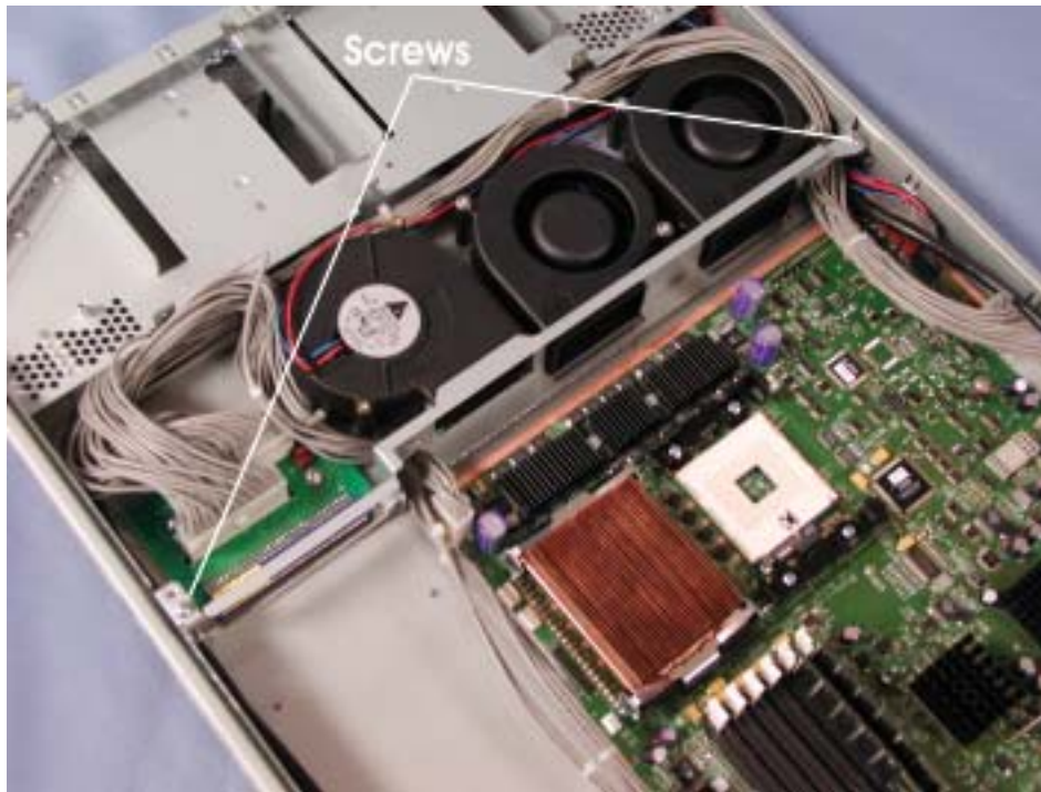
Figure 3-35. Fan Assembly Bracket
