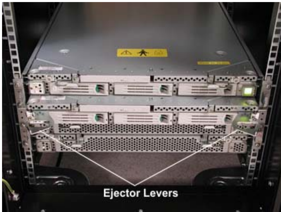
Figure 3-23. I/O Enclosure Ejection Levers
