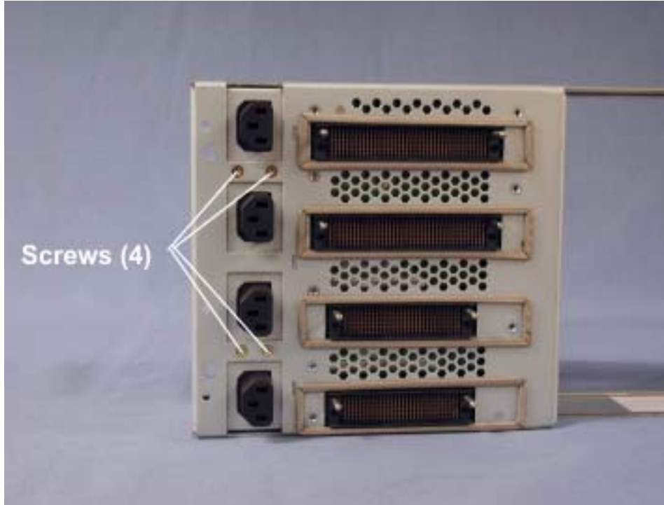
Figure 4-82. AC Distribution Screws
