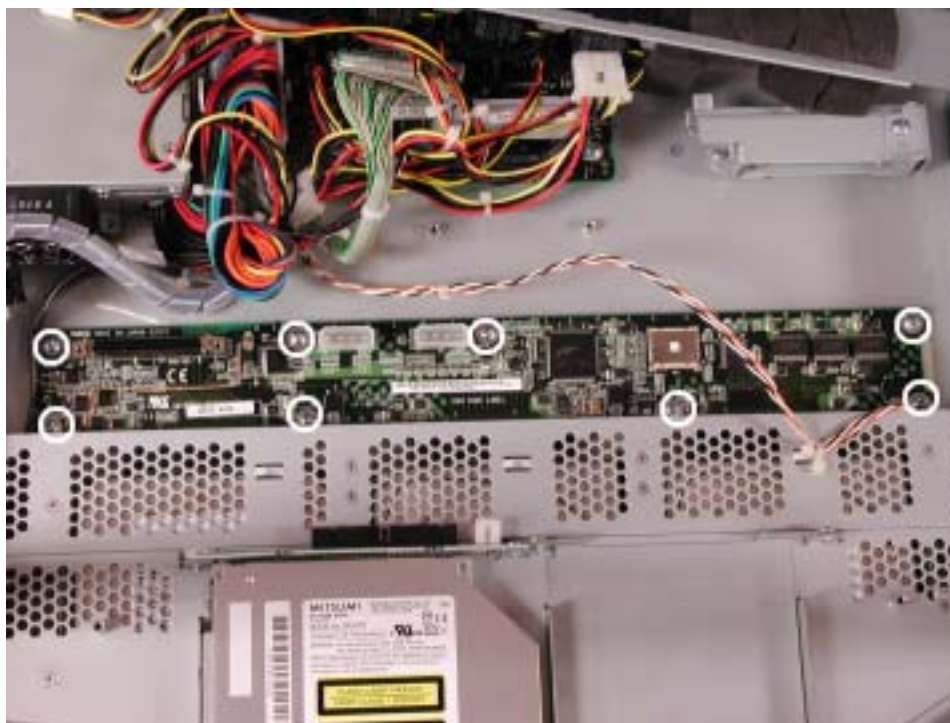
Figure 4-67. SCSI Backplane Screws
