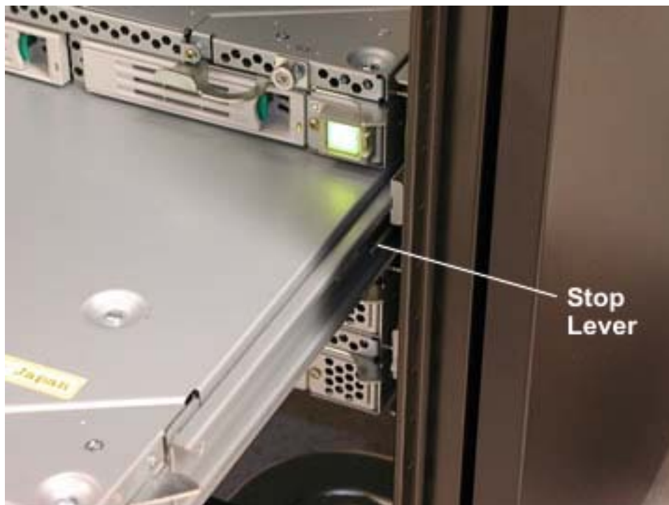
Figure 3-24. Removing I/O Enclosure
