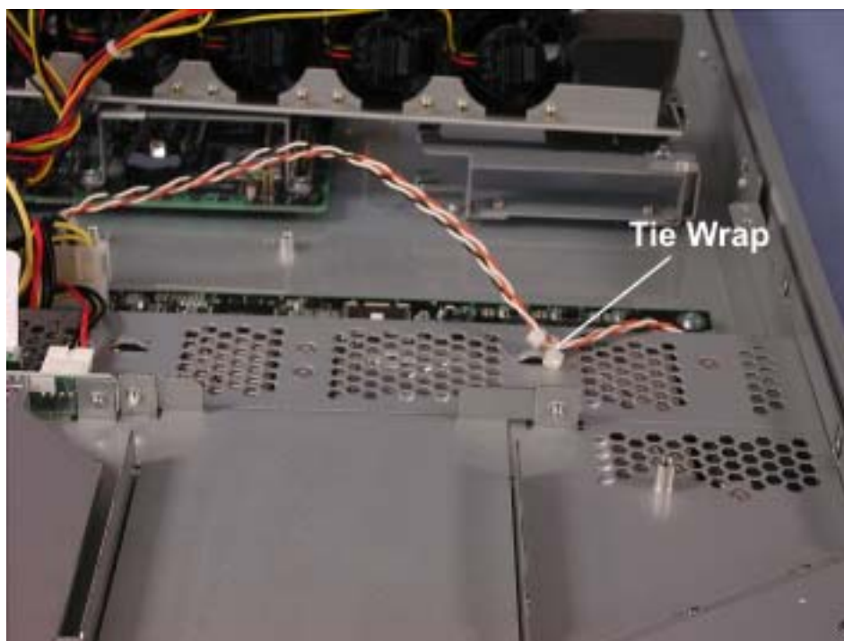
Figure 4-73. Power Switch Cable Tie Wrap
