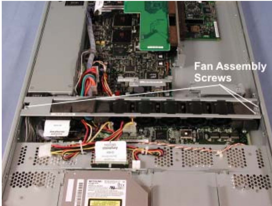
Figure 4-52. Fan Assembly Screws
