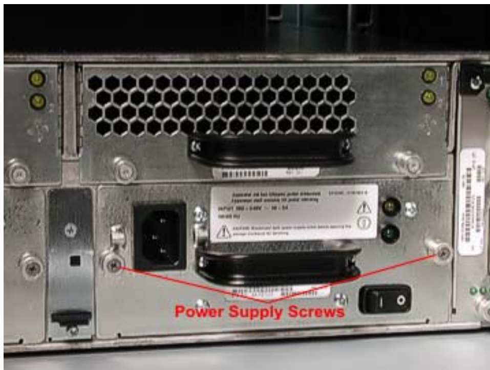
Figure 3-63. Power Supply Screws.
