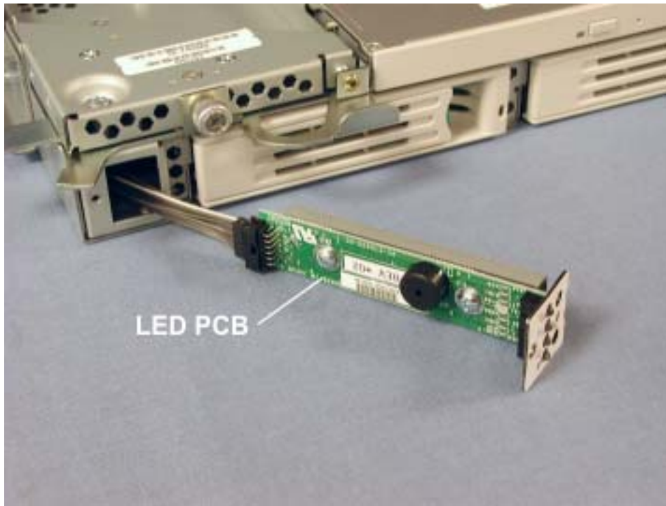
Figure 4-71. Removing LED PCB and Cable
