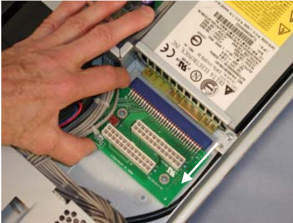
Figure 4-26. Removing the Power Connector Board
