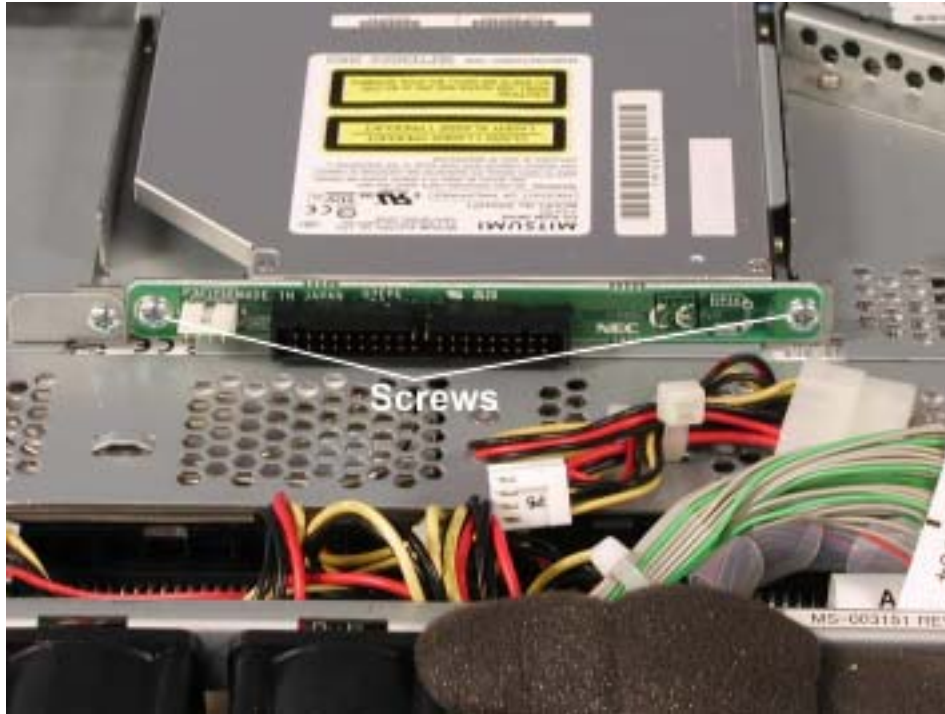
Figure 5-34. CD-ROM Interface Board Screws
