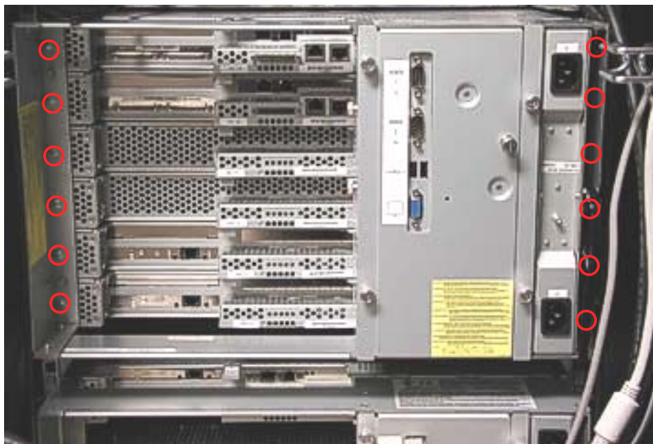
Figure 4-29. Backplane Assembly Screws
