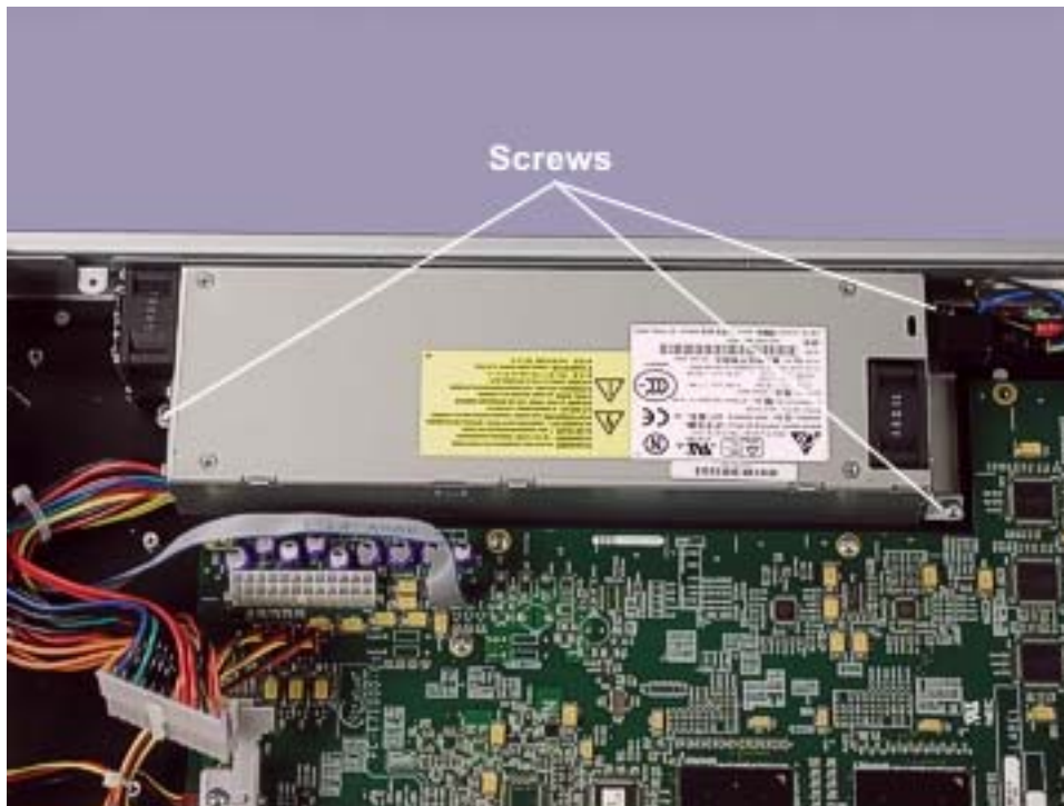
Figure 4-71. Power Supply Screws
