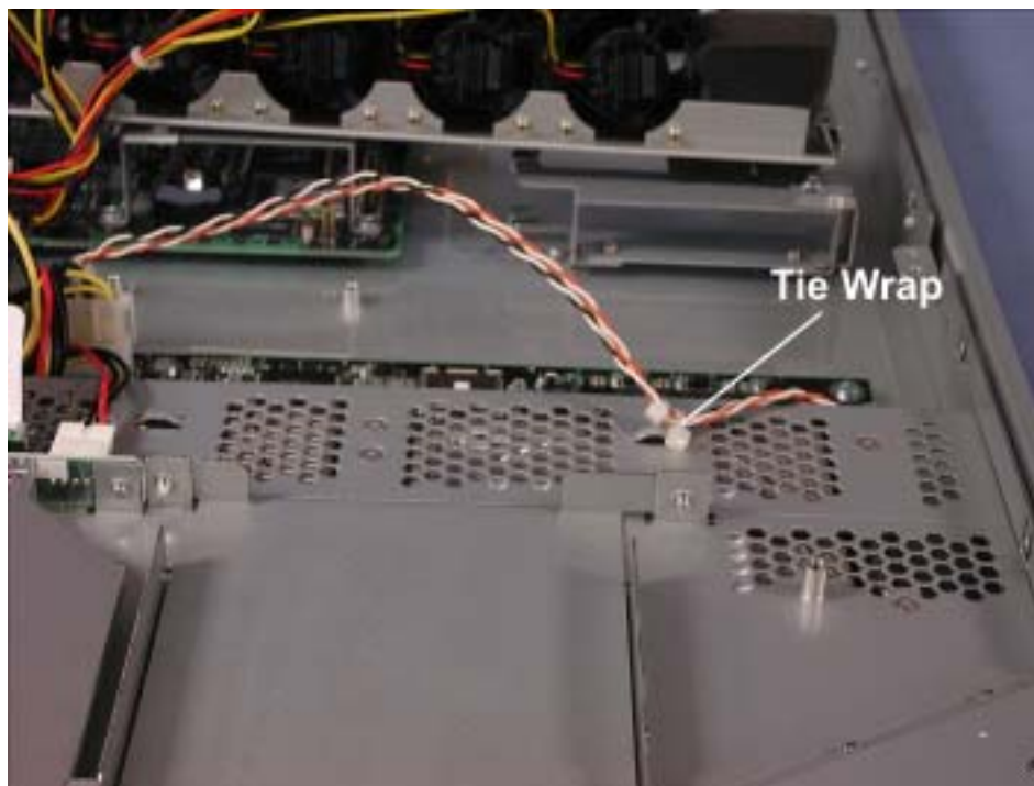
Figure 4-40. Power Switch Cable Tie Wrap
