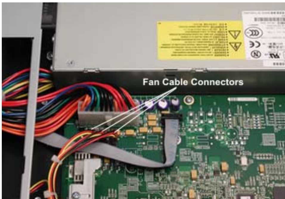
Figure 3-47. Fan Assembly Power Cable Connections
