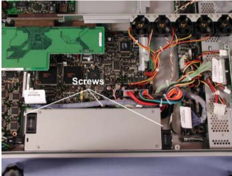
Figure 4-18. Power Supply Screws
