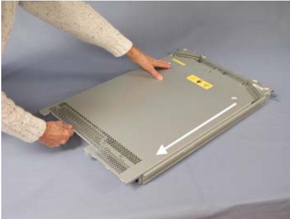
Figure 3-26. Removing Enclosure Cover
