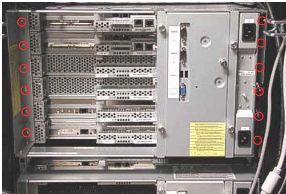
Figure 3-57. Backplane Assembly Screws
