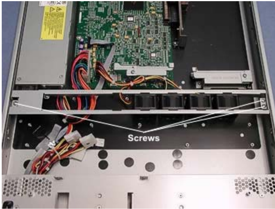
Figure 4-21. Fan Assembly Screws
