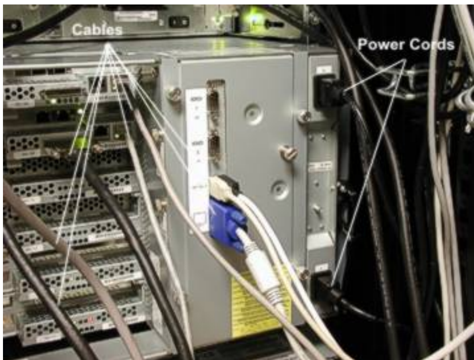
Figure 4-89. Power Cord and Cable Connections at Rear of Cabinet
