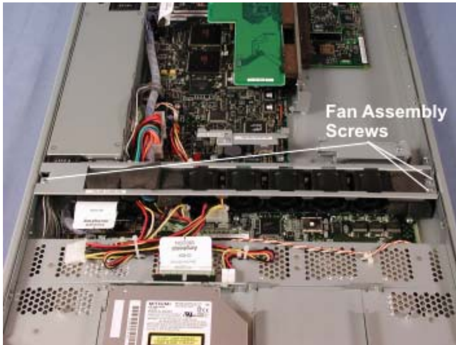
Figure 4-57. Fan Assembly Screws
