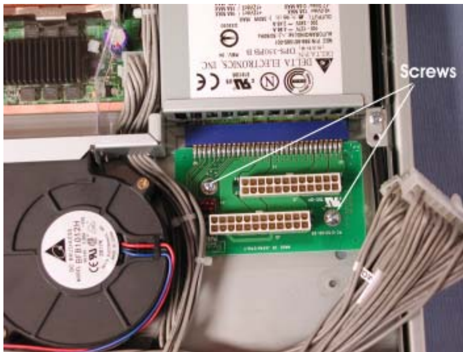
Figure 5-20. Power Connector Board Screws
