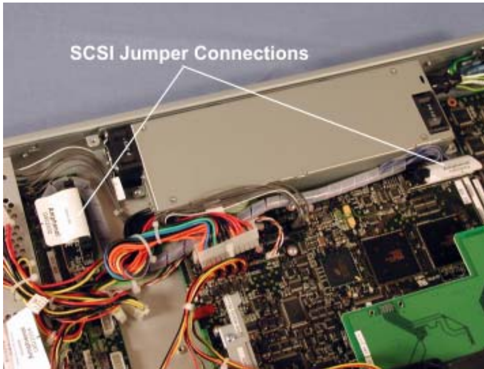
Figure 5-46. Ultra160 SCSI Jumper Connections
