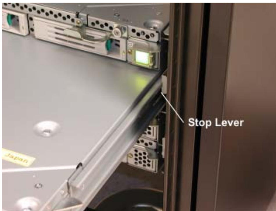
Figure 3-24. I/O Enclosure Stop Lever
