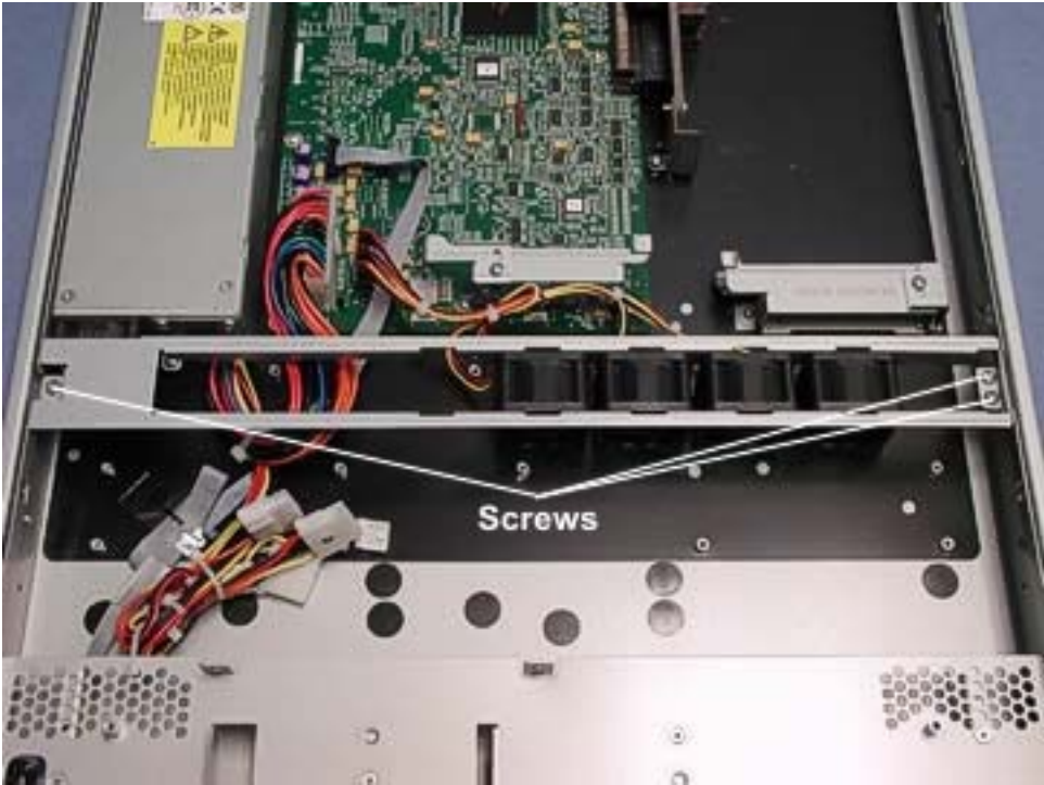
Figure 4-84. Fan Assembly Screws
