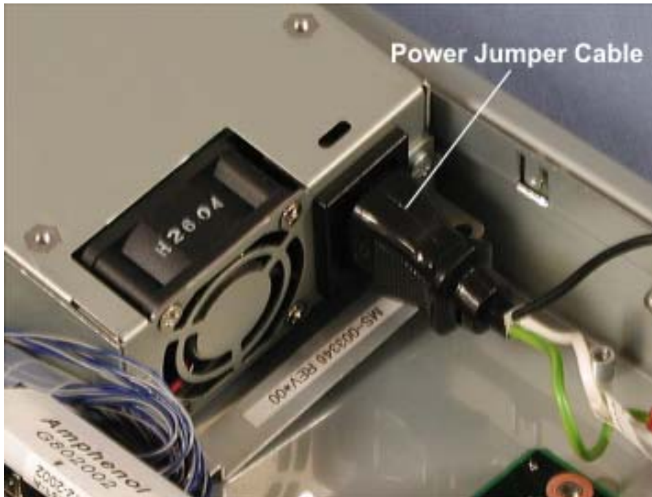
Figure 4-38. Power Jumper Cable Connection
