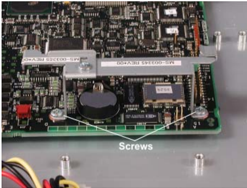
Figure 4-46. Stabilizing Bracket Screws
