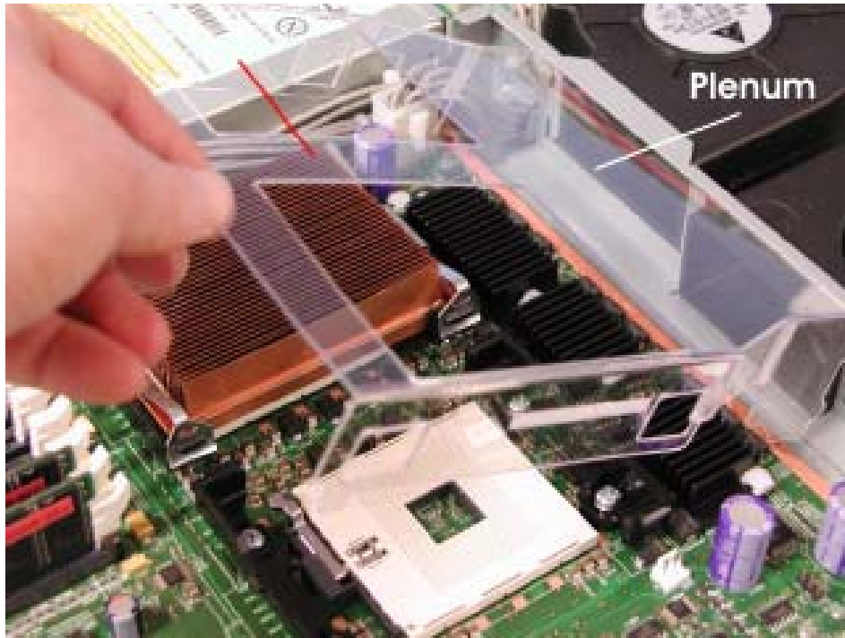
Figure 5-4. Removing the Plastic Plenum
