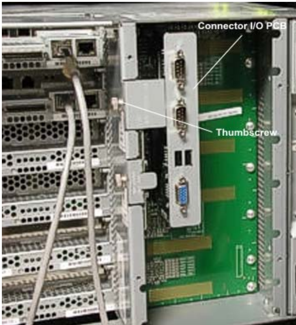
Figure 3-51. Connector I/O PCB Screw
