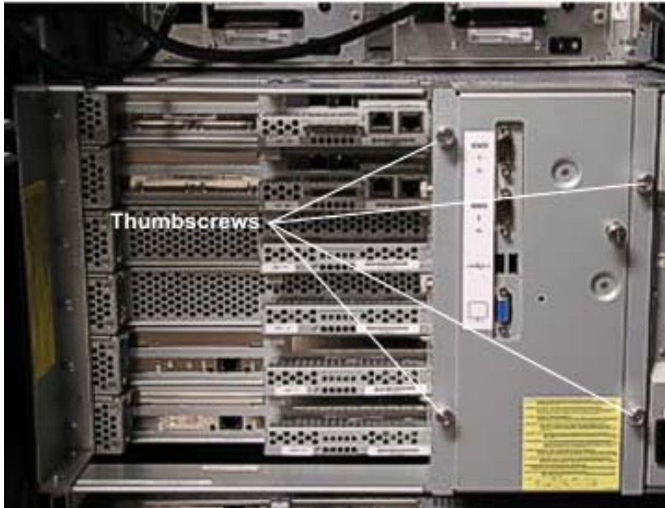
Figure 3-50. Backplane Cover Plate Screws
