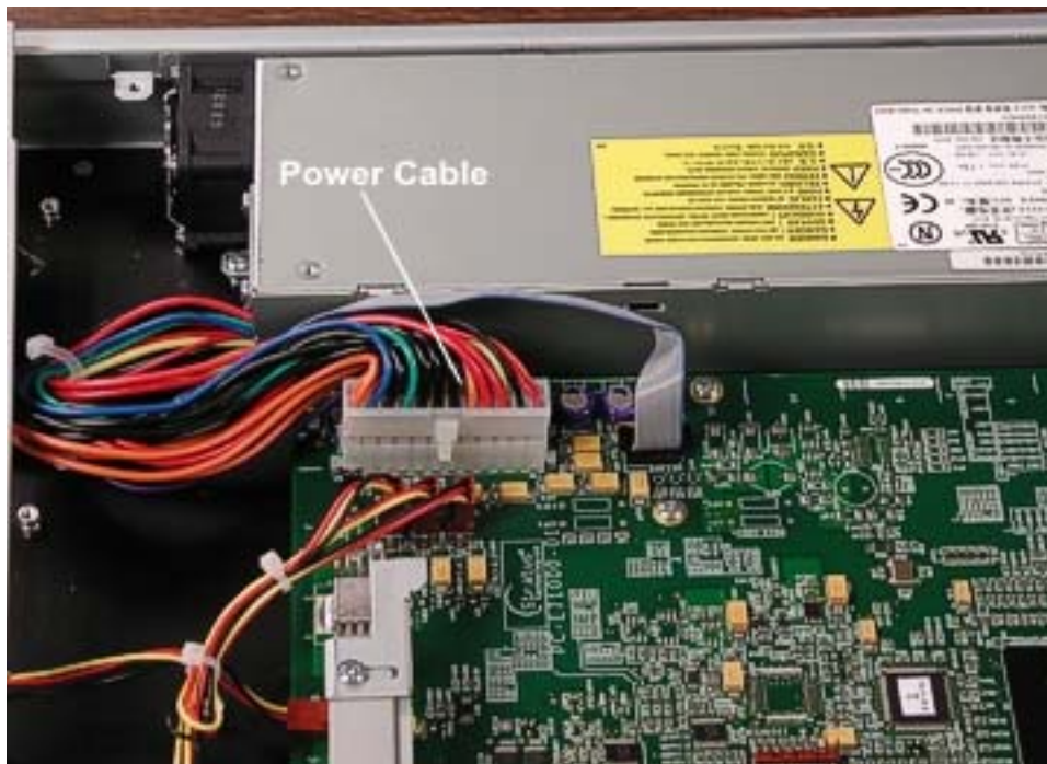
Figure 4-22. Power Cable Connection at Expansion I/O Board
