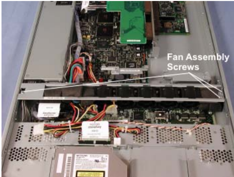
Figure 4-68. Fan Assembly Screws
