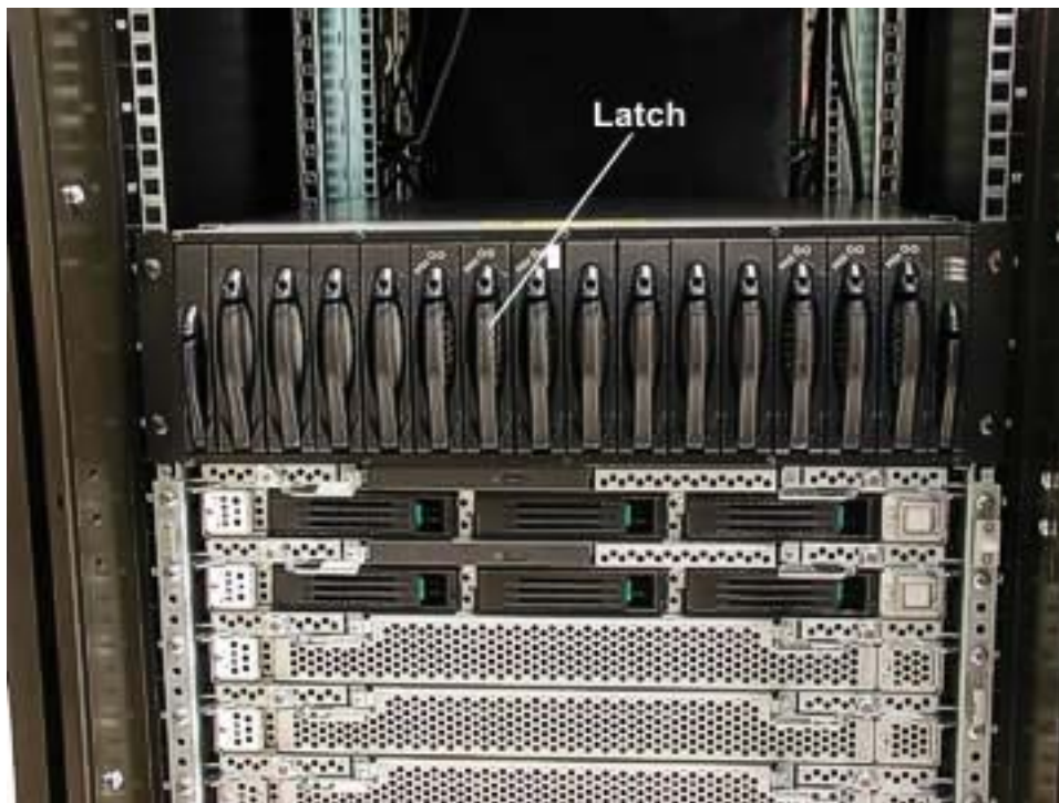
Figure 3-62. SCSI Disk Drive Latching Arm
