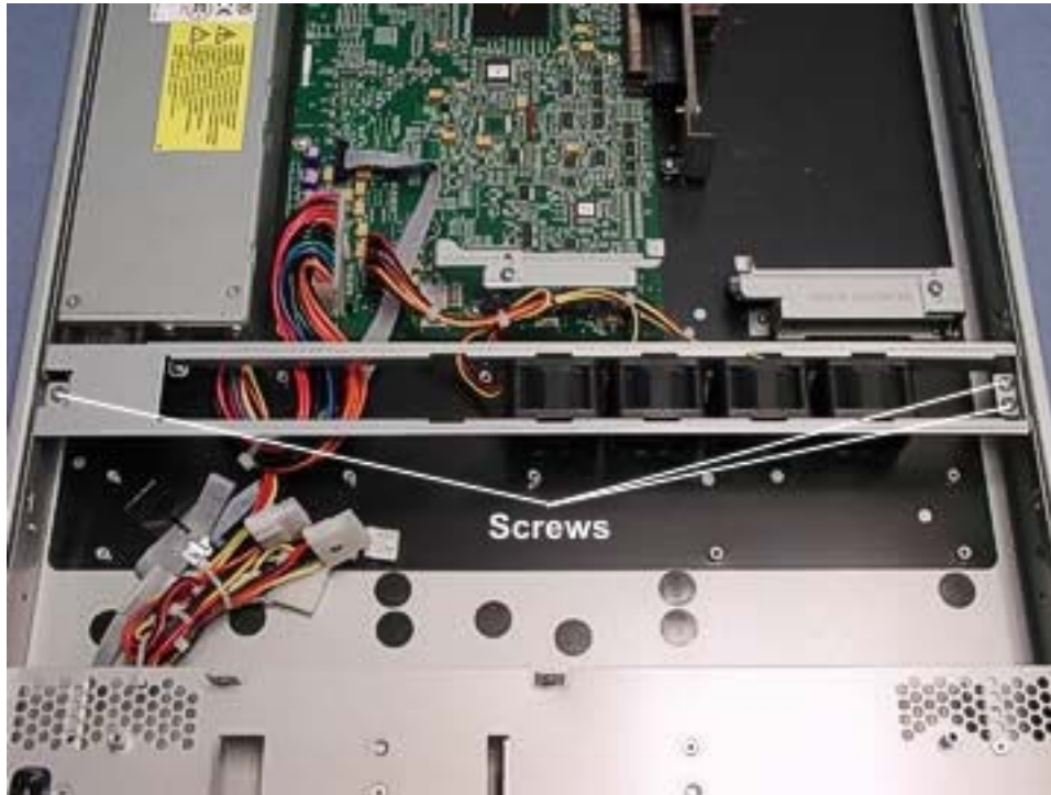
Figure 4-68. Fan Assembly Screws
