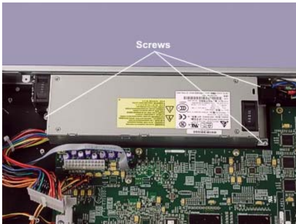
Figure 4-24. Power Supply Screws
