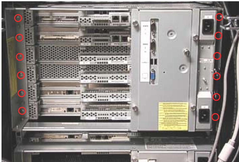
Figure 3-54. Backplane Assembly Screws
