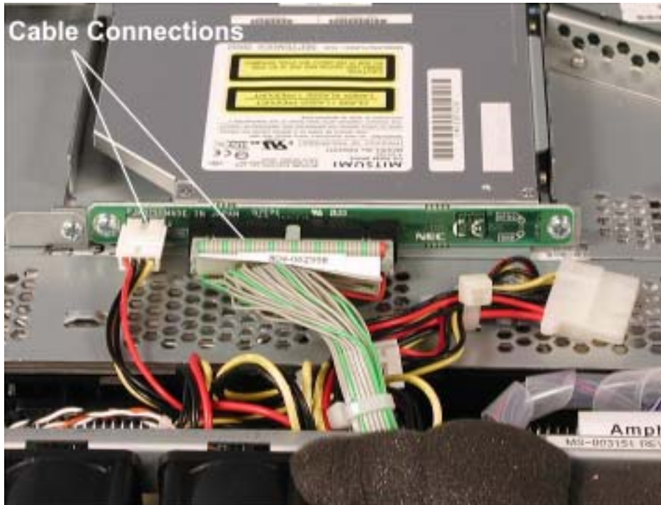
Figure 4-50. CD-ROM Interface Board Cables
