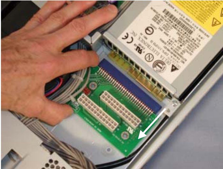
Figure 5-21. Removing the Power Connector Board
