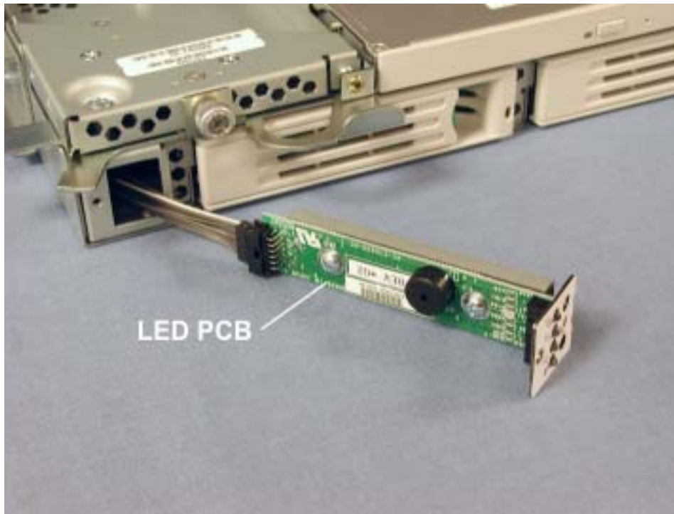
Figure 5-54. Removing LED PCB and Cable
