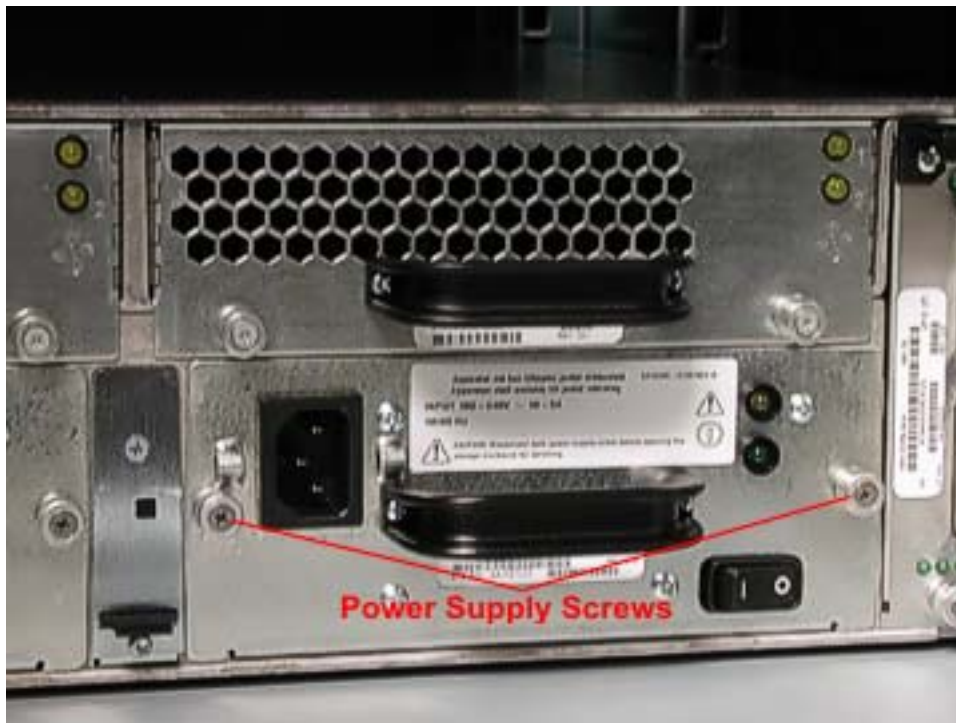
Figure 3-67. Power Supply Screws.
