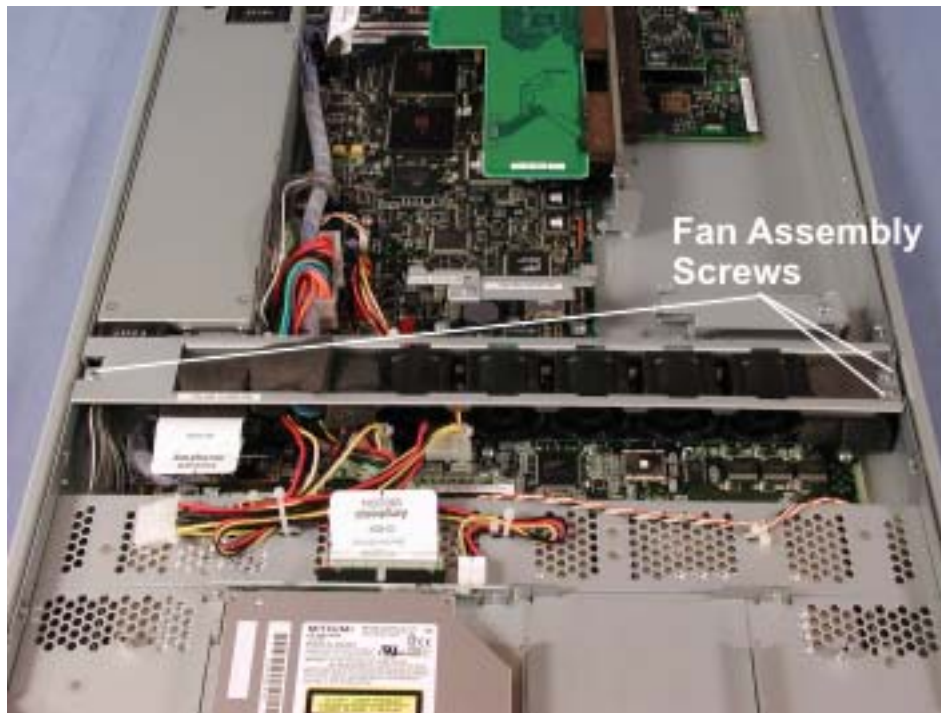
Figure 4-72. Fan Assembly Screws
