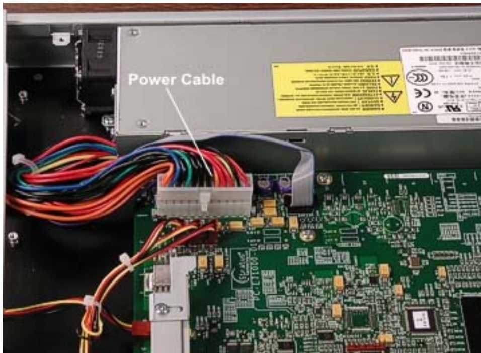
Figure 4-69. Power Cable Connection at Expansion I/O Board
