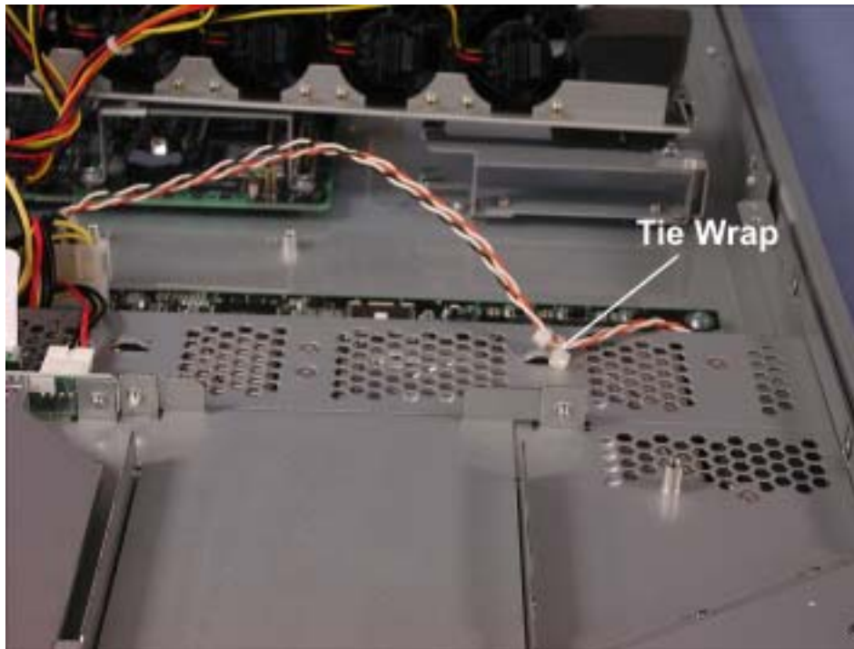
Figure 5-23. Power Switch Cable Tie Wrap
