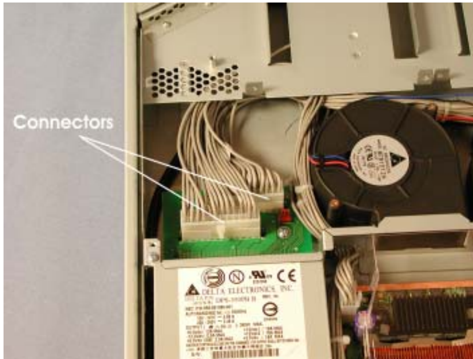
Figure 5-19. Power Connector Board Connectors
