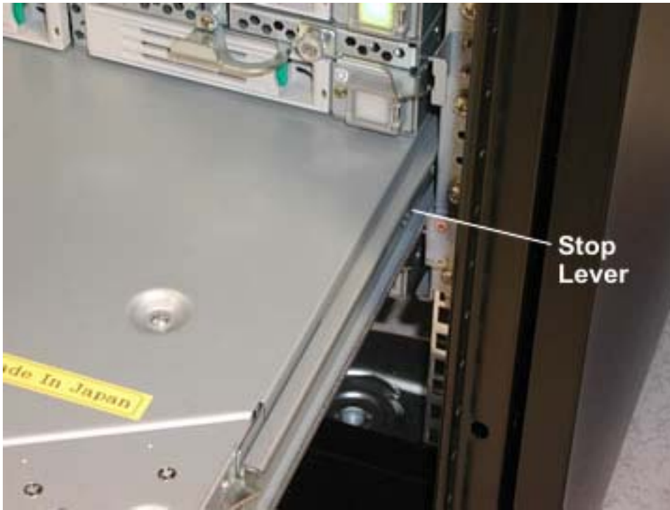
Figure 3-13. CPU Enclosure Stop Lever
