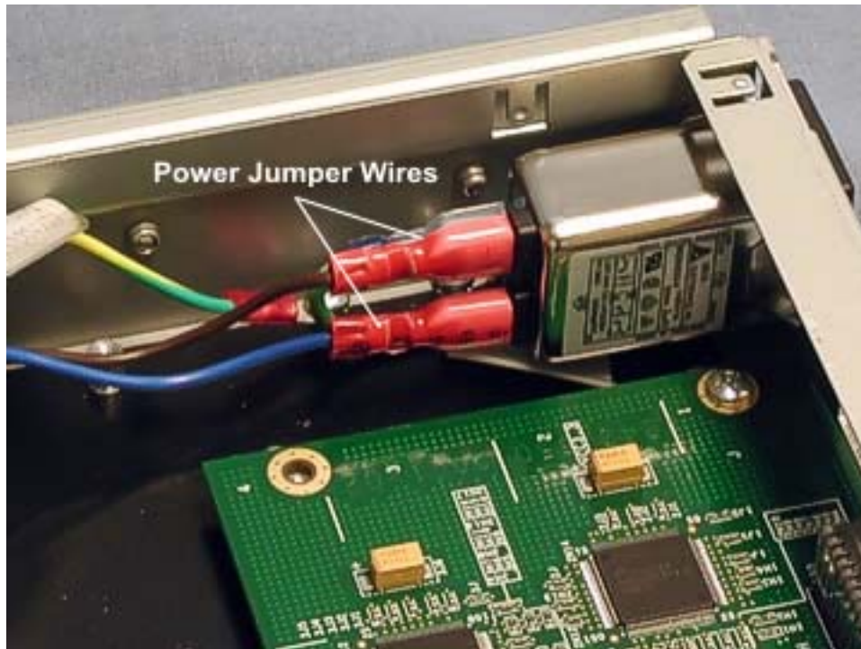
Figure 4-87. Power Jumper Cable Wires at AC Inlet
