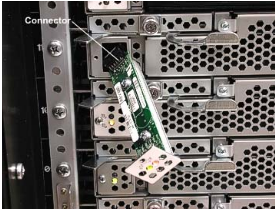
Figure 3-33. Removing LED PCB
