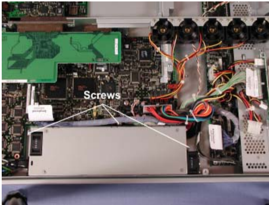
Figure 4-36. Power Supply Screws
