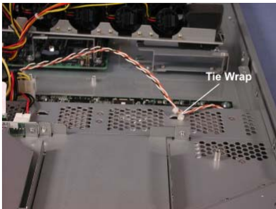
Figure 4-73. Power Switch Cable Tie Wrap
