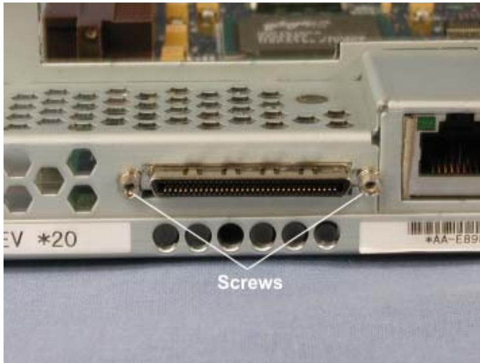
Figure 5-31. External SCSI Connector Screws
