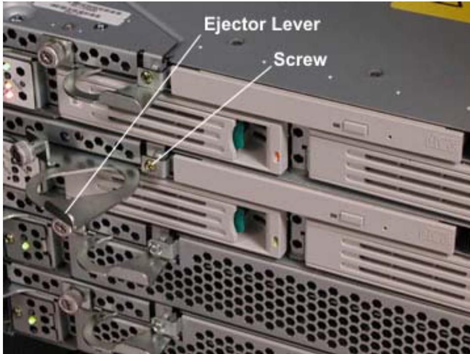
Figure 3-44. I/O Enclosure Ejector Lever and CD-ROM Screw
