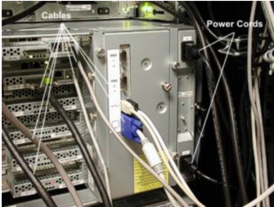
Figure 4-27. Power Cord and Cable Connections at Rear of Cabinet
