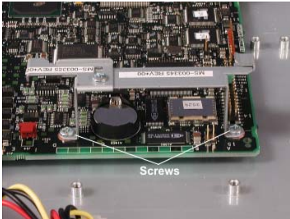
Figure 5-29. Stabilizing Bracket Screws
