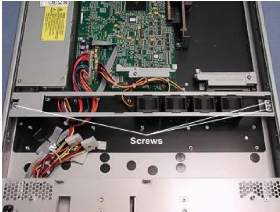
Figure 3-46. Fan Assembly Screws
