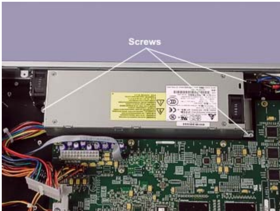
Figure 4-86. Power Supply Screws
