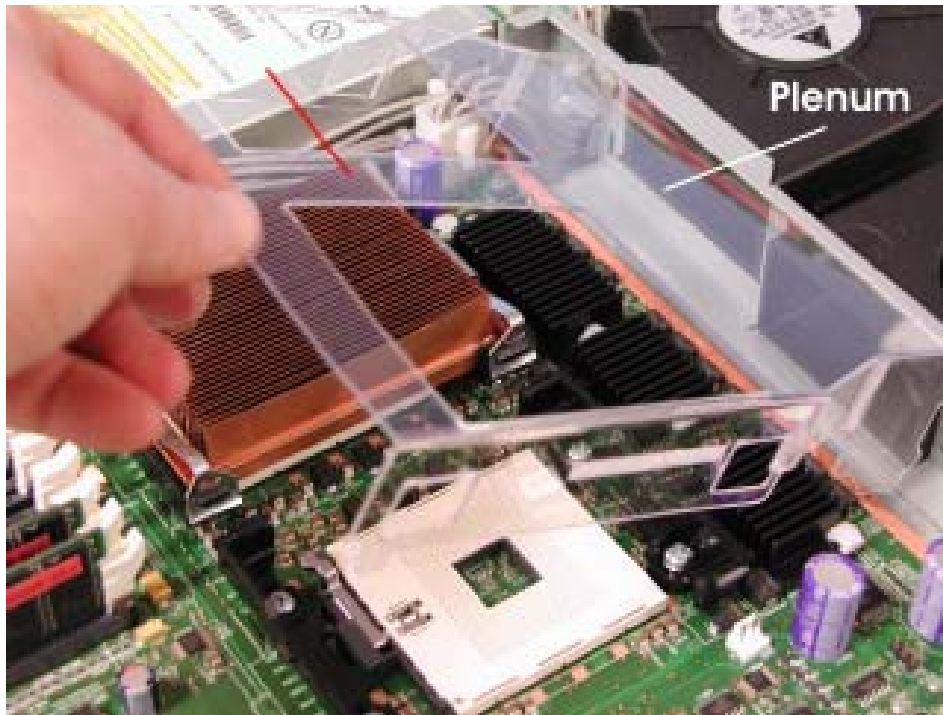
Figure 4-9. Removing the Plastic Plenum
