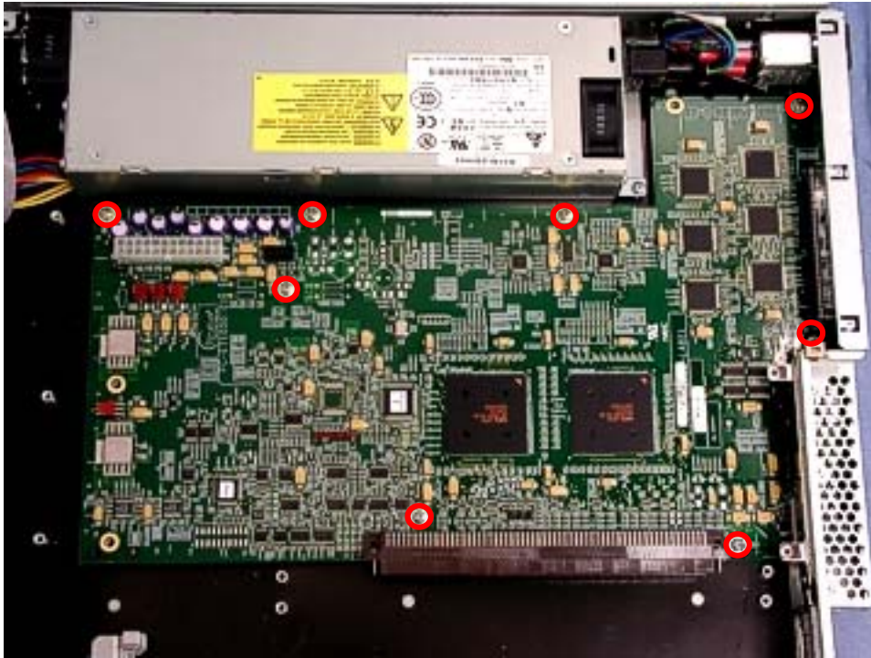
Figure 4-79. Expansion I/O Board Screws
