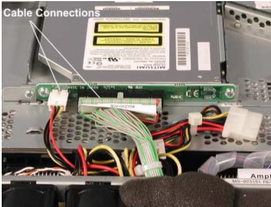
Figure 5-25. CD-ROM Interface Board Cables
