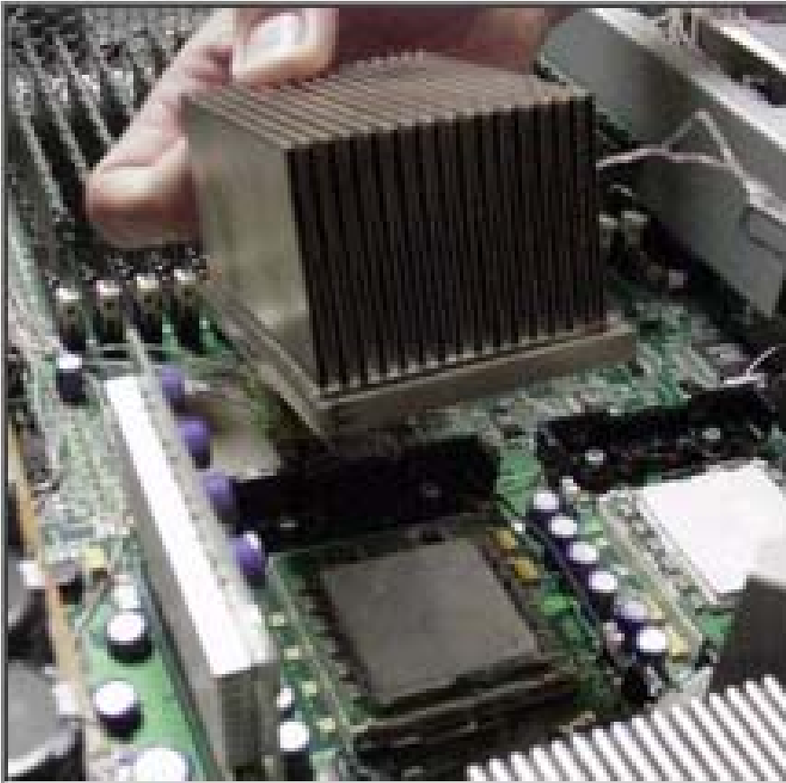
Figure 5-10. Replacing Heat Sink
