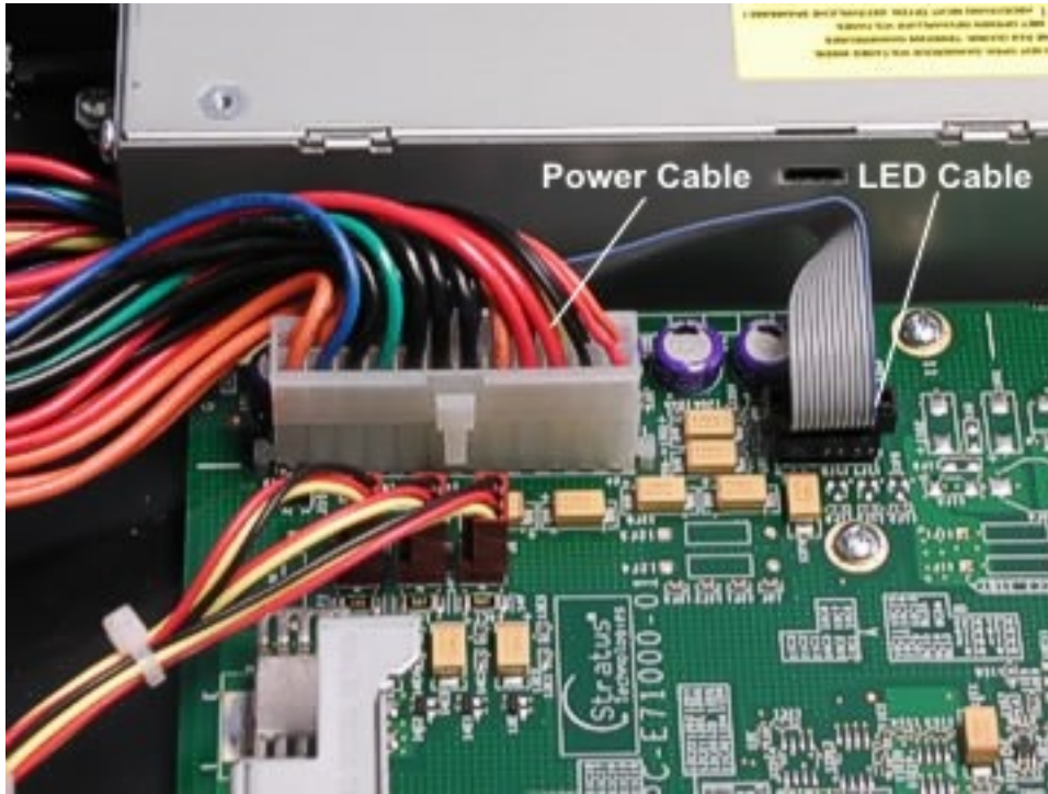
Figure 5-27. Power Cable and LED Cable Connections at I/O Expansion Board
