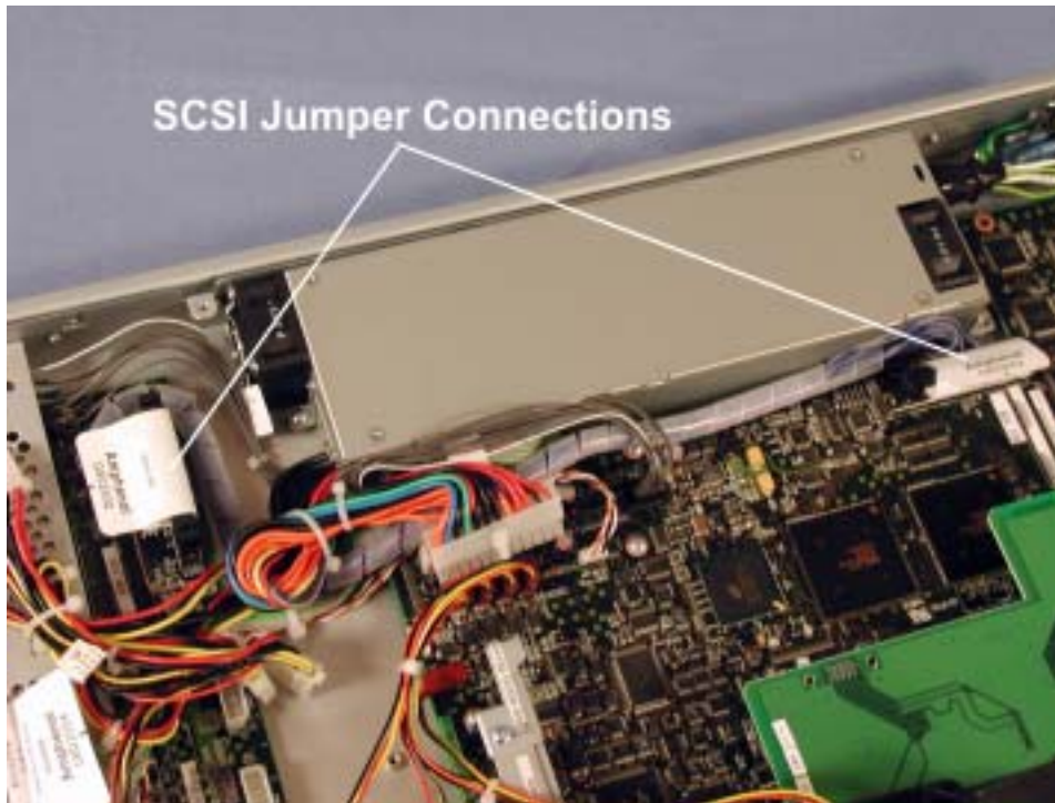
Figure 5-64. Ultra160 SCSI Jumper Connections
