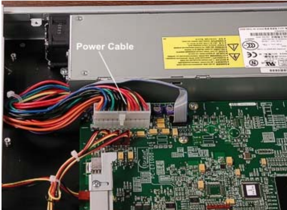
Figure 4-20. Power Cable Connection at Expansion I/O Board
