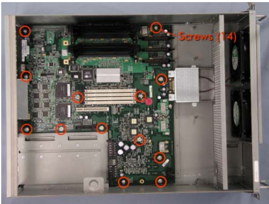
Figure 3B-3. Motherboard Screws
