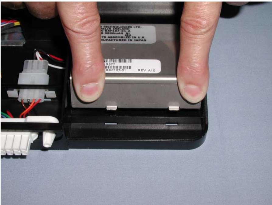
Figure 4B-33. Releasing the Battery (R2)
