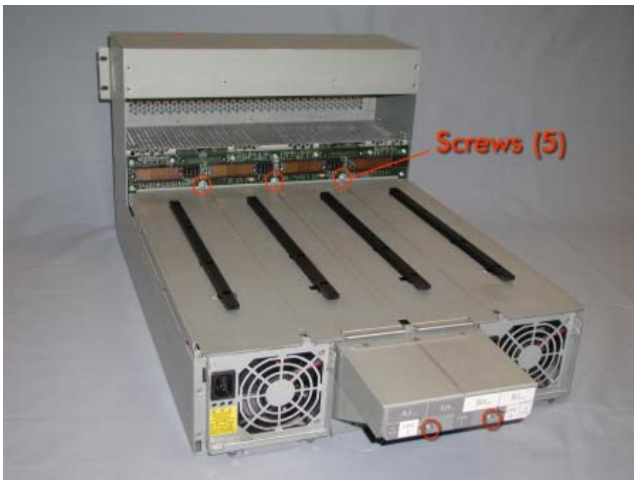
Figure 3B-7. LVDS I/O Power and Distribution Board Cover Screws
