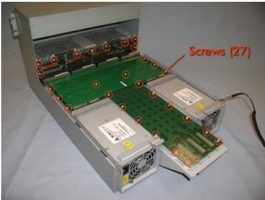
Figure 3B-9. LVDS I/O Power and Distribution Board Screws
